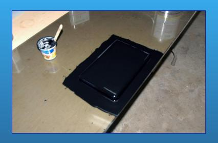
ProSet Tooling Epoxy Applied with to desired thickness. This may require two coats especially on vertical surfaces.
