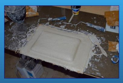
After the last layer is worked down then the 'feet' are applied. Small diameter PVC pipe was used for this.
